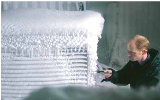
Climatic chambers simulate all possible operating conditions
