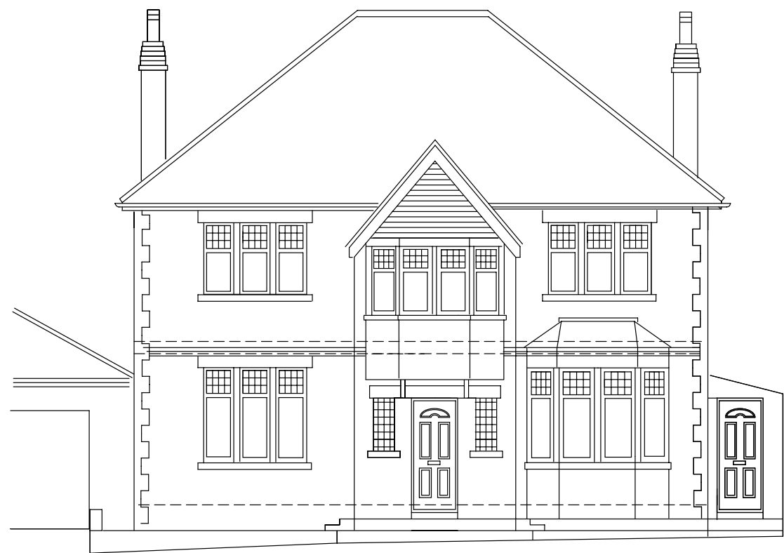
EXISTING FRONT ELEVATION
