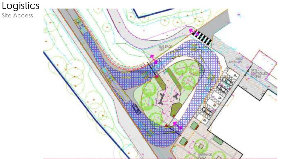
27 Pisch FOLMITS: Swept pots analysis to indicate the pots of beick vehicle construction. This swept path alones the antibulated vehicle traveling around central bland and the path require noid driving across any outer living of the road lowaut is kerts 7 cen perking spaces. This indicates the vehicle' trailer would impact on the rentral bland at two conters, path das des the whole nound would be required without any other bistructions.
