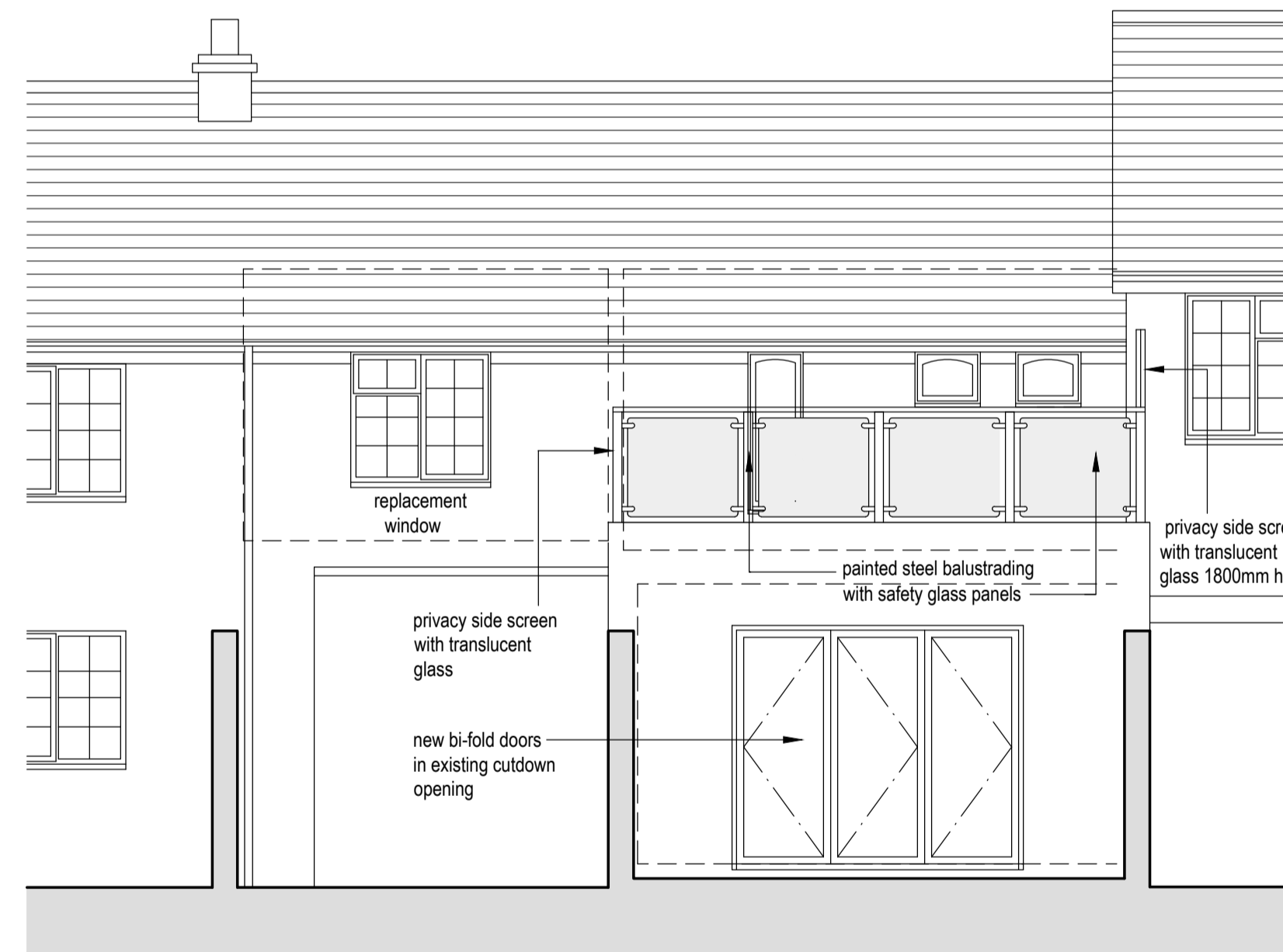
proposed south elevation - 1 : 50
