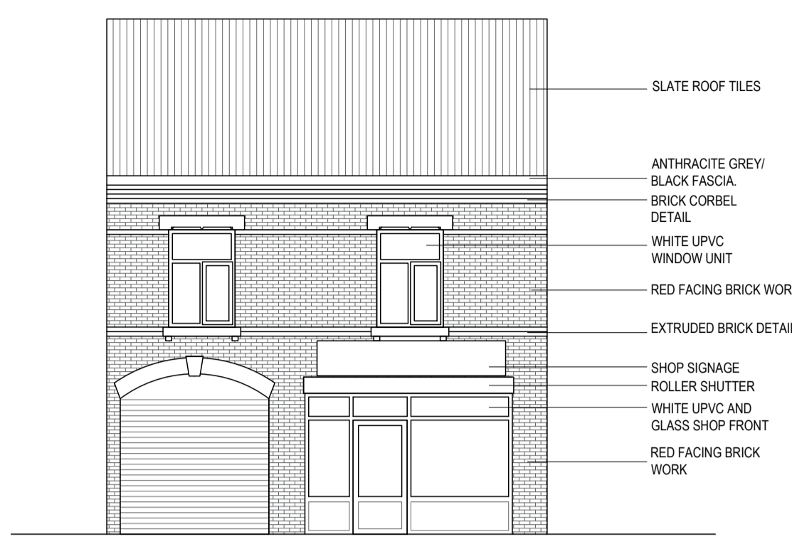
EXISTING FRONT ELEVATION SCALE 1/100
