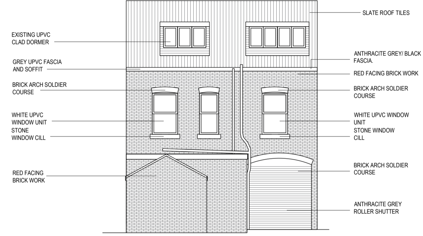
EXISTING REAR ELEVATION SCALE 1/100
