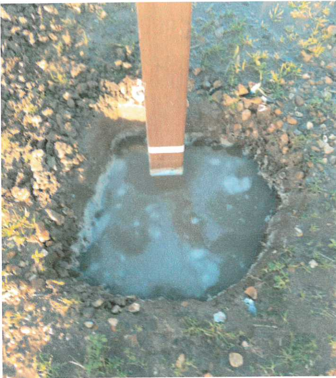
FIGURE 7: Time 14-54 - Level of water at 225mm (START)
