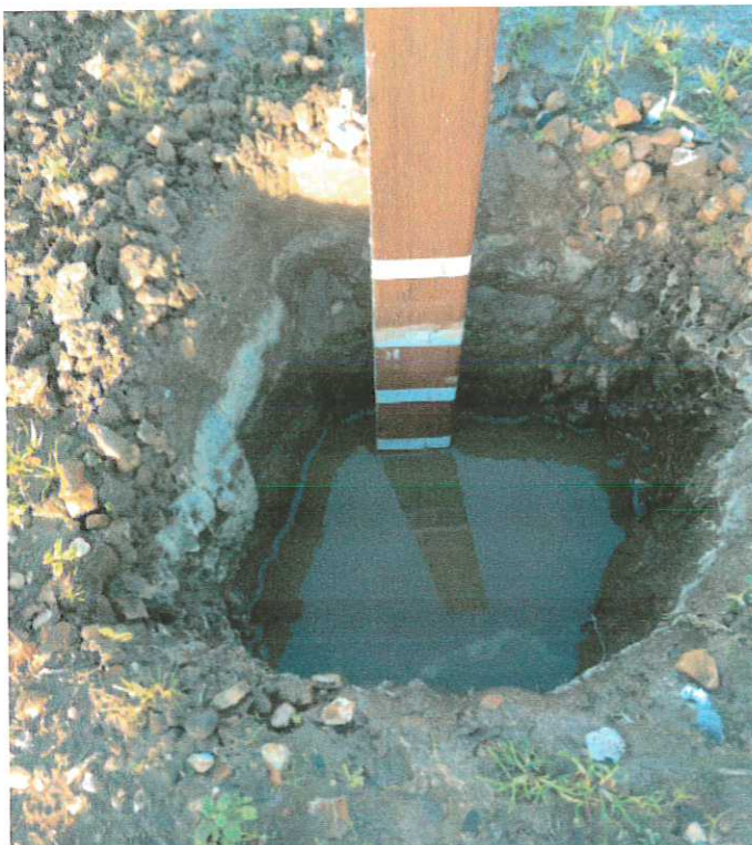
E 9: Time 14-56 - Level of water at 75mm (END)
