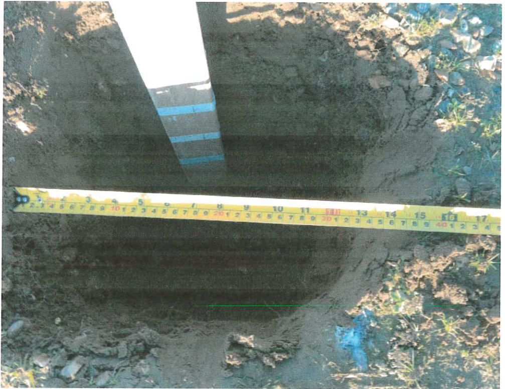
FIGURE 3: Time 14-40 - Test pit width is 300mm
