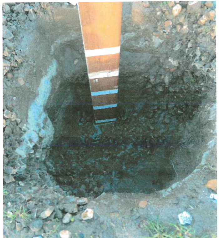
FIGURE 10: Time 14-59 - Water drained from test pit
