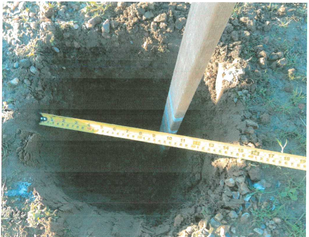
FIGURE 4: Time 14-41 - Test pit length is 300mm
