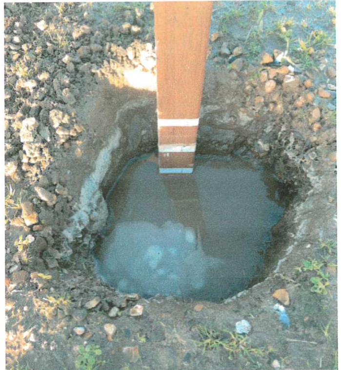
FIGURE 8: Time 14-55 - Level of water at 150mm
