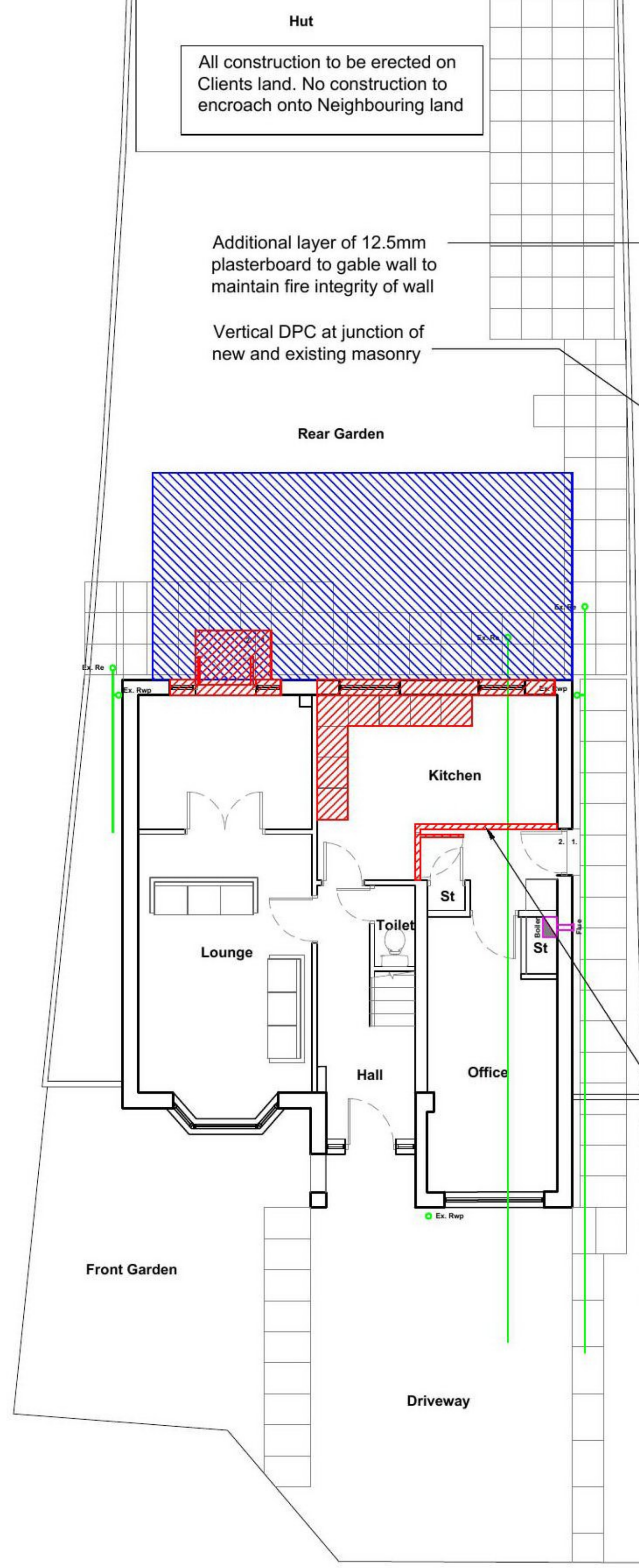
EXISTING GROUND FLOOR PLAN SCALE 1:100
