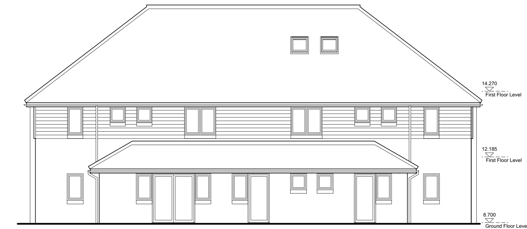
NORTH (Rear) ELEVATION: as existing 1:100
