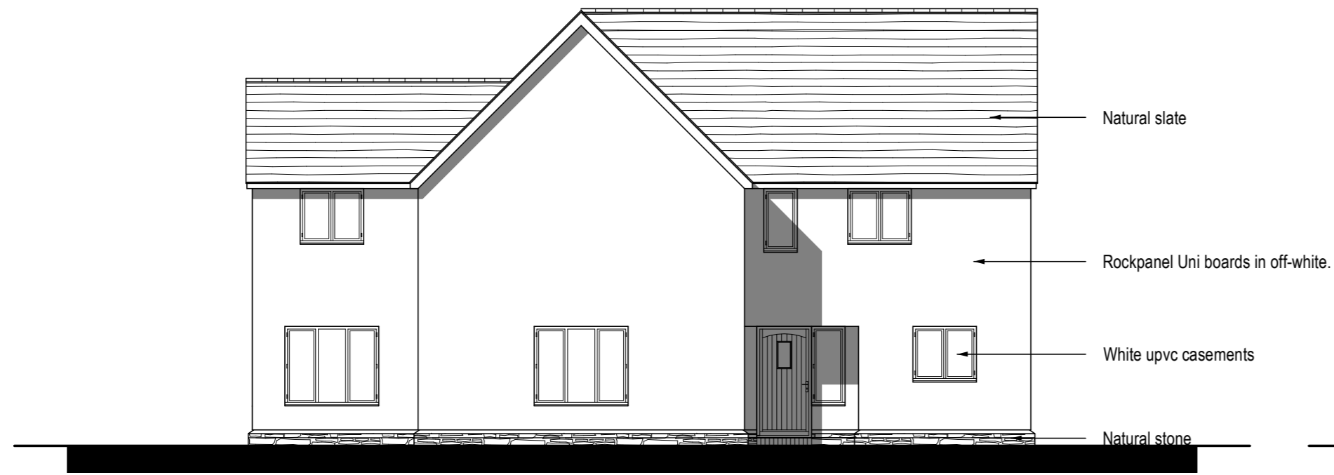
FRONT (NORTH) ELEVATION
