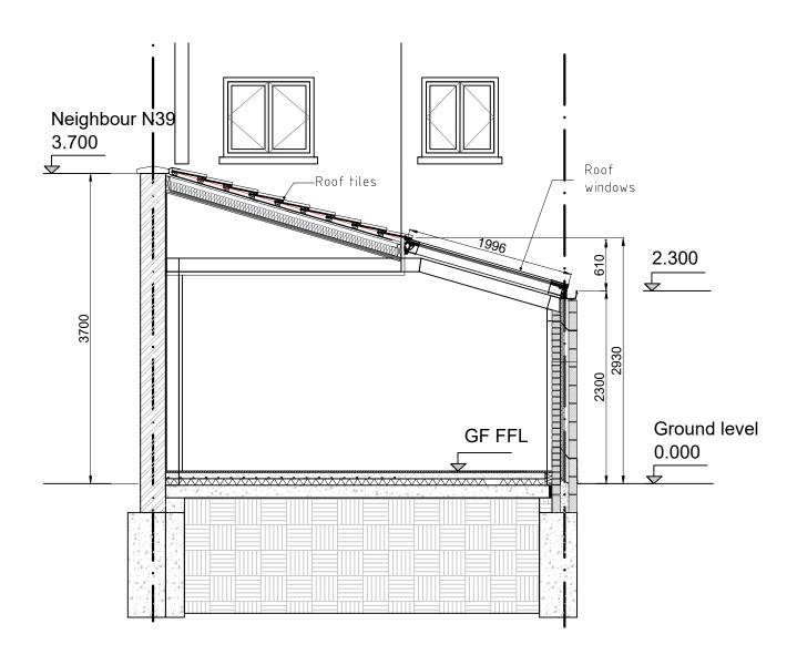
Note: New extension roof height to start at the extension height at N39 and drop dawn to 2.3m above ground level at party wall with N35.
