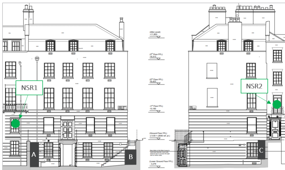
Figure 4: Proposed plant units location and nearest NSRs
