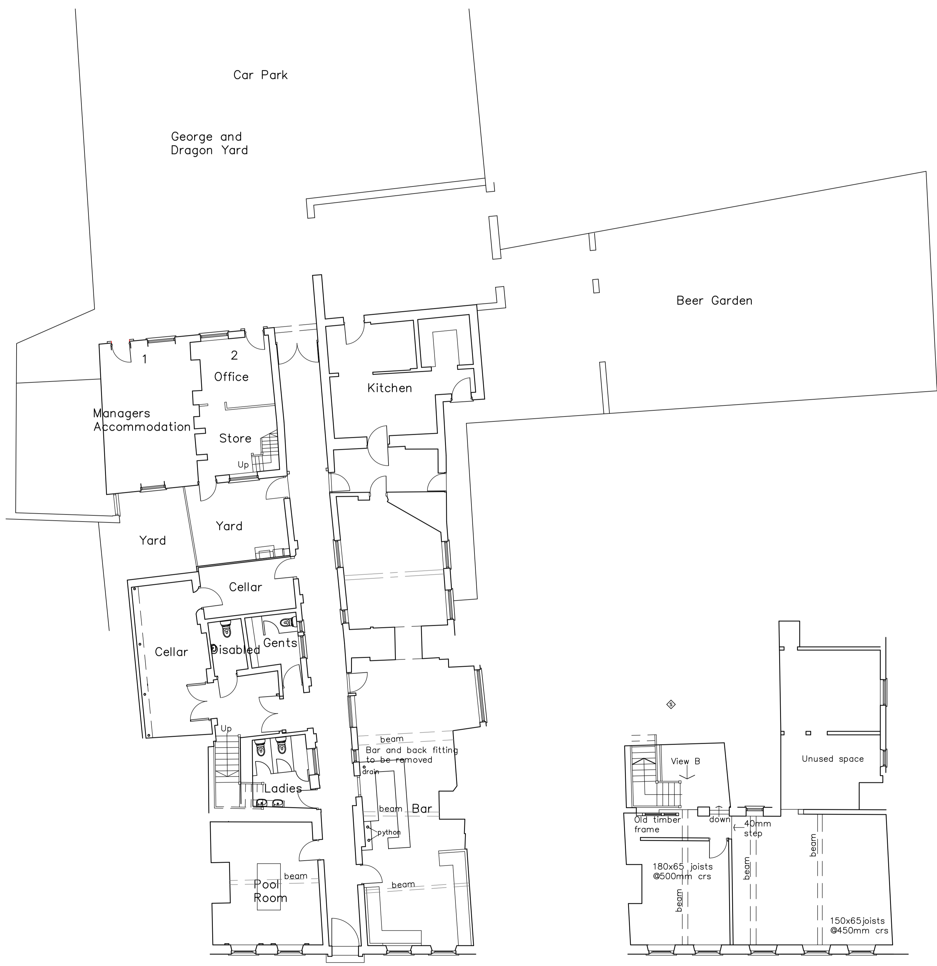
Highgate Existing Ground Floor Plan Scale Bar (1:100) 0 5m
