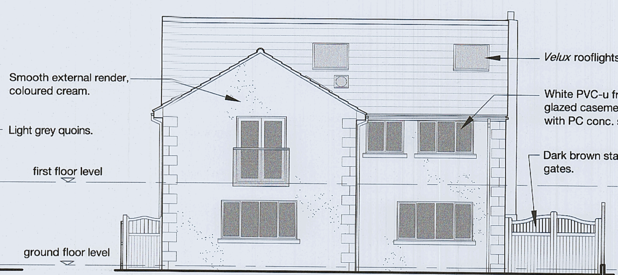
FRONT ELEVATION 1:100 SOUTH EAST
