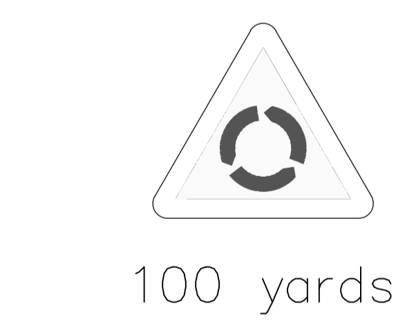
ROUNDABOUT SIGN (DIA 510) WITH SUPPLEMENTARY DISTANCE PLATE (DIA 572).
