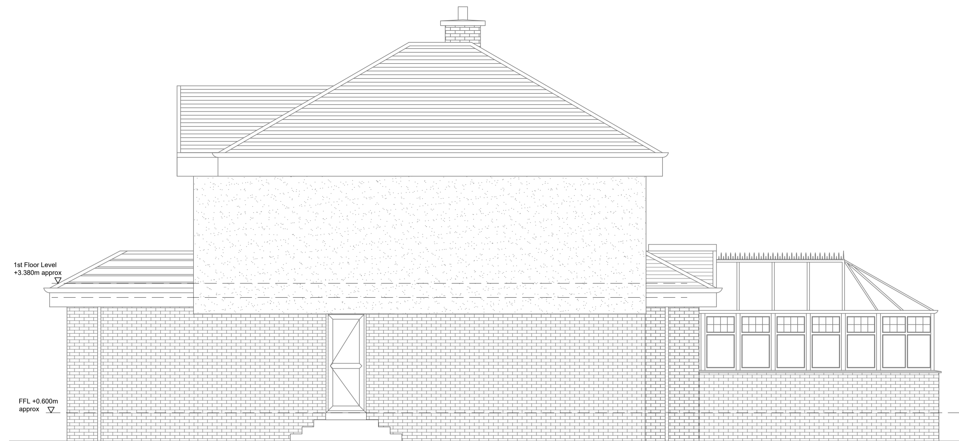
EXISTING SIDE (EAST) ELEVATION Scale 1:50
