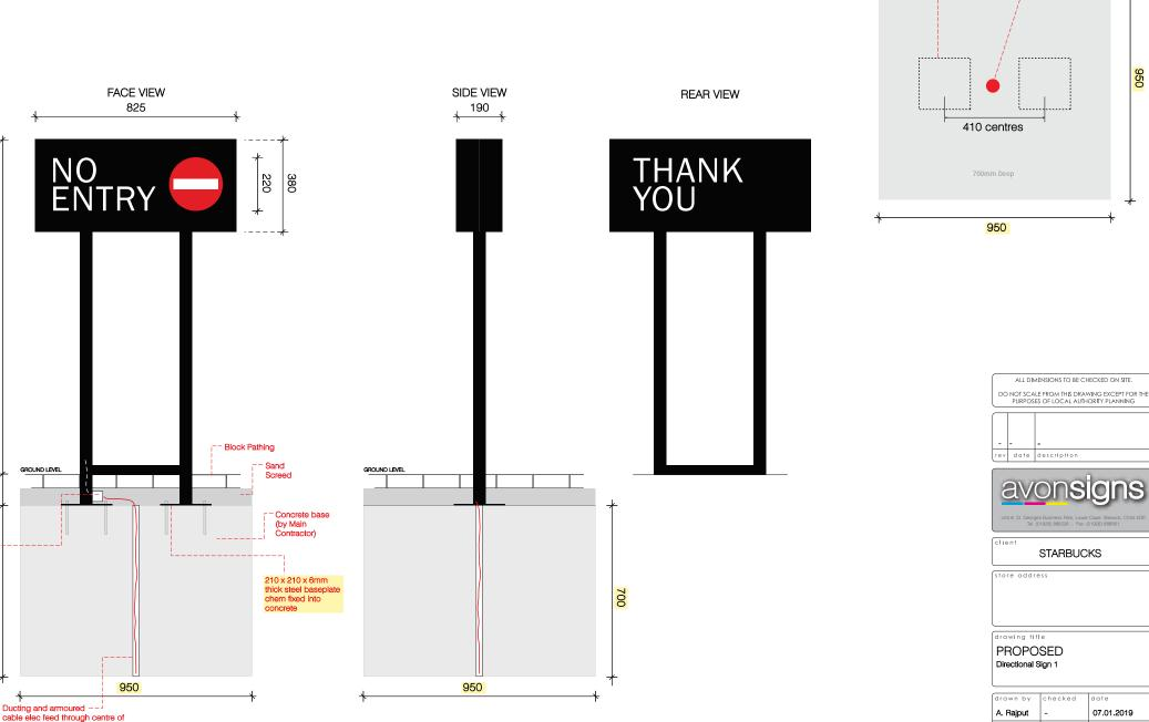
cable elec feed through centre of concrete pad (by Main Contractor).
