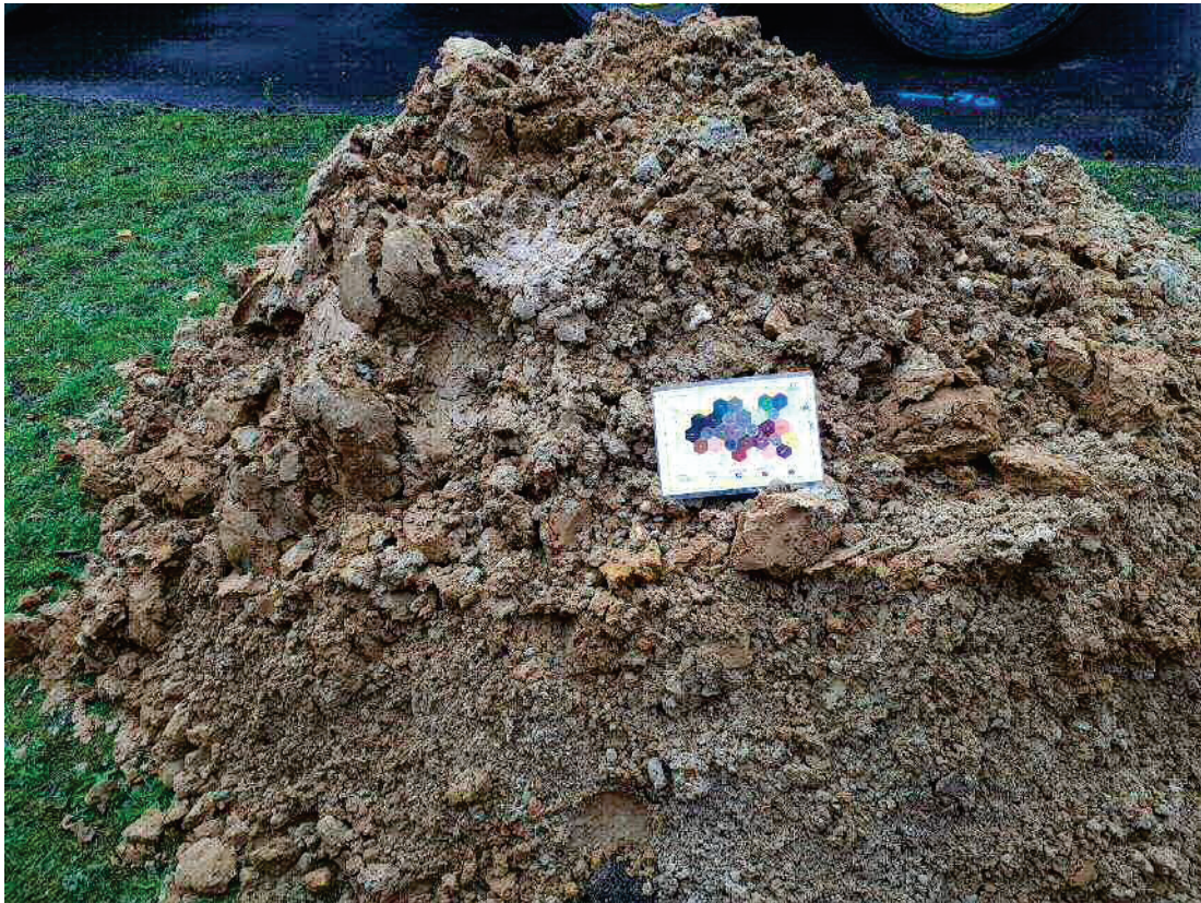
Photograph 3: Arisings encountered at TP01.
