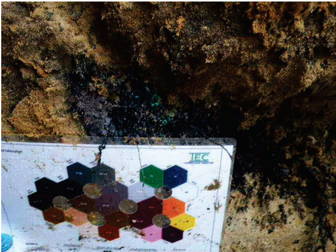
Photograph 4: Encountered materials from TP01. Recorded black silty sandy lens with occasional to rare green speckles and rootlets from 0.30m to 0.45m..
