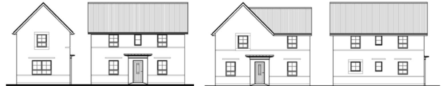
Example of true dual aspect dwellings utilised within the development to enable active streetscenes and natural surveillance over all public spaces.
