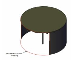
2) Once the front section is opened up appropriately, the roof sheeting is to be removed using the shear followed by the internal roof structural steel purlins and the "t-beam" section.
