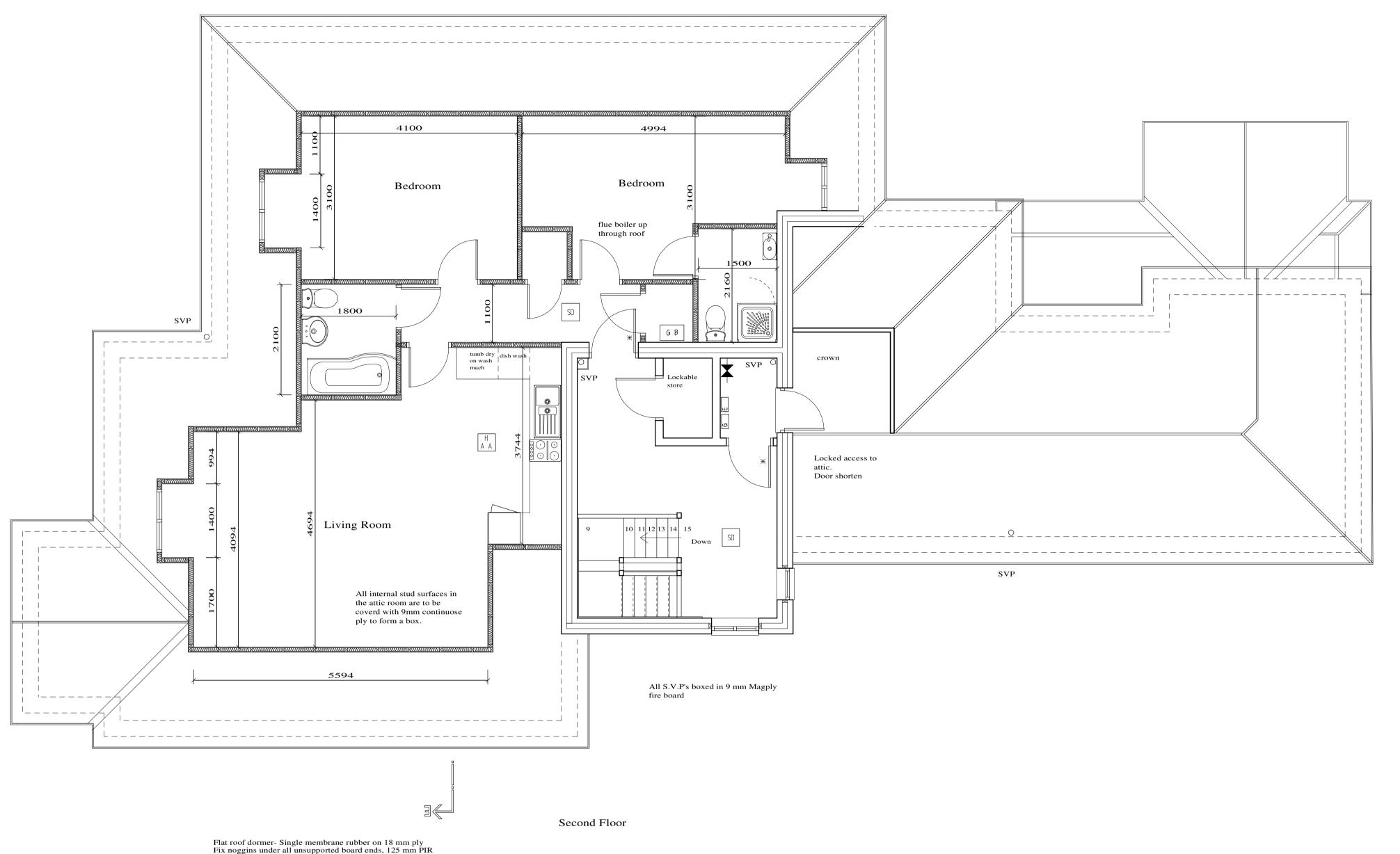
Flat roof dormer- Single membrane rubber on 18 mm ply
