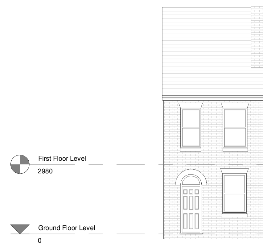
1 Existing Front Elevation 1 : 100
