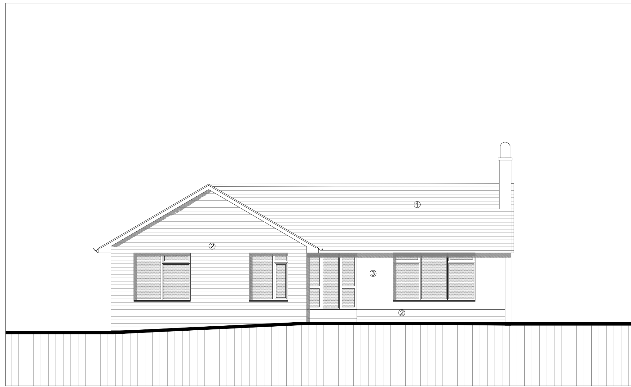
EXISTING NORTH ELEVATION 1:100
