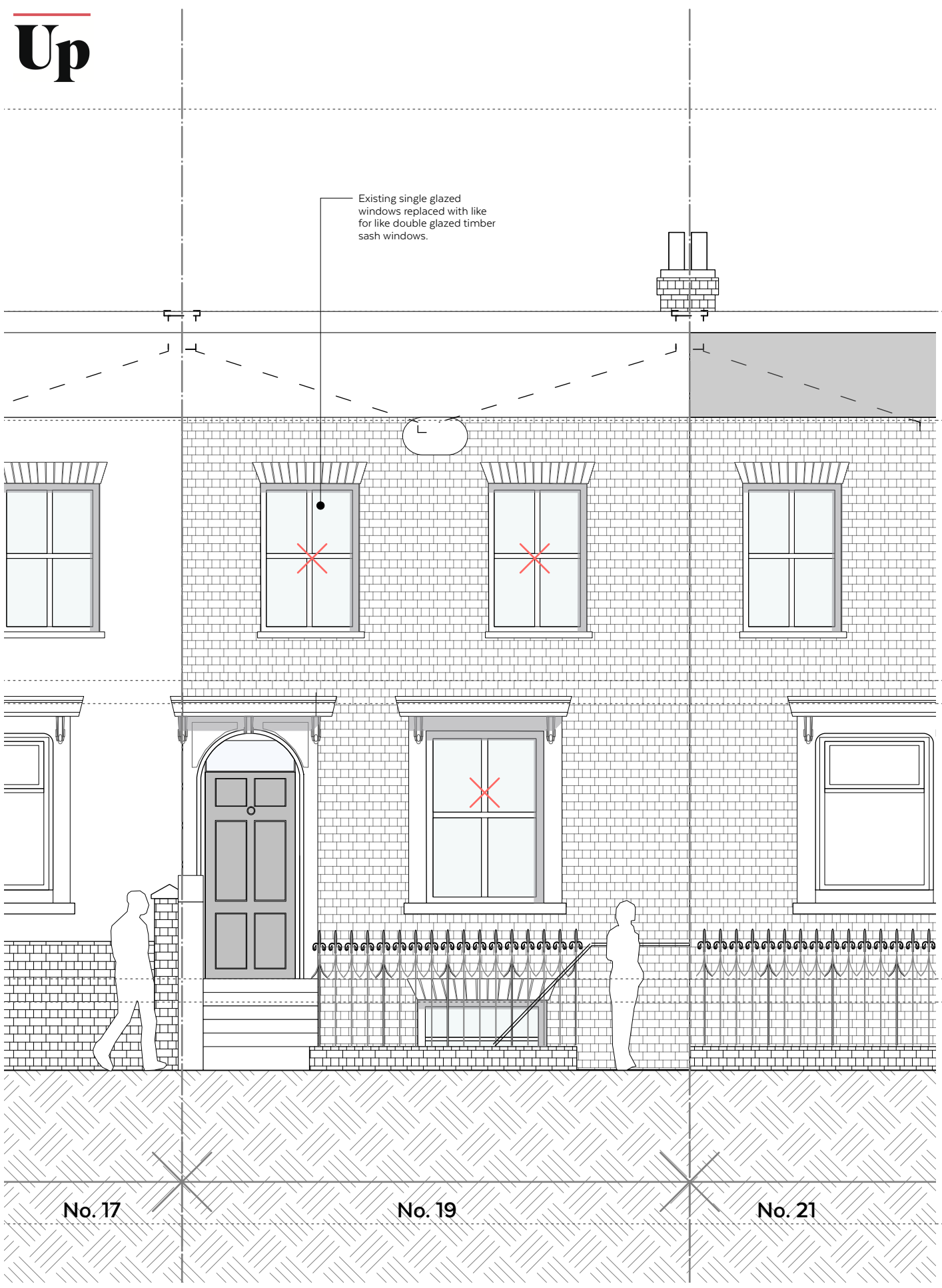
Existing Front Elevation - 1:50 @ A3
