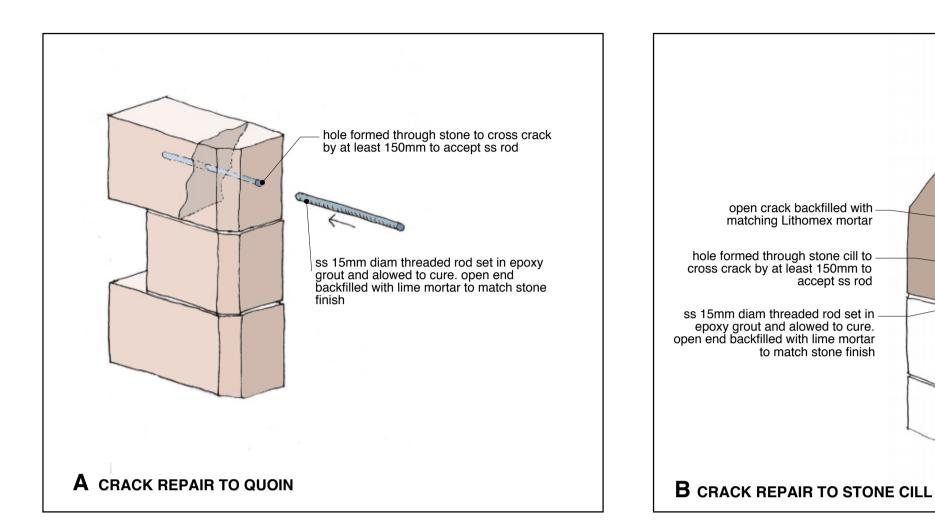
**NOTE:** exact type of stitching to be agreed on site with CA. Where threaded dowels used they must be stainless and should bed into the stone at least 200mm either side of crack. In some cases a full stone indent may be required
