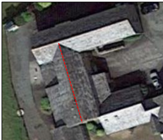
Figure 5. Aerial showing location of temporary internal partition, ensuring the void [and access points] remain undisturbed during construction
