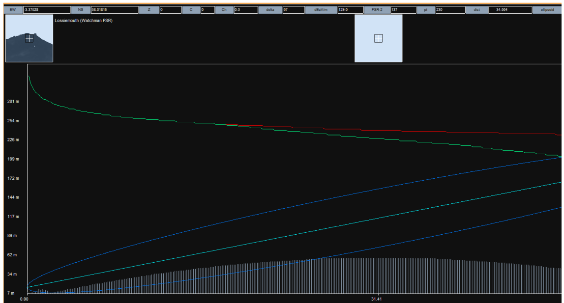
Figure 2 RAF Lossiemouth PSR LOS and terrain elevation profile to WTG T1
