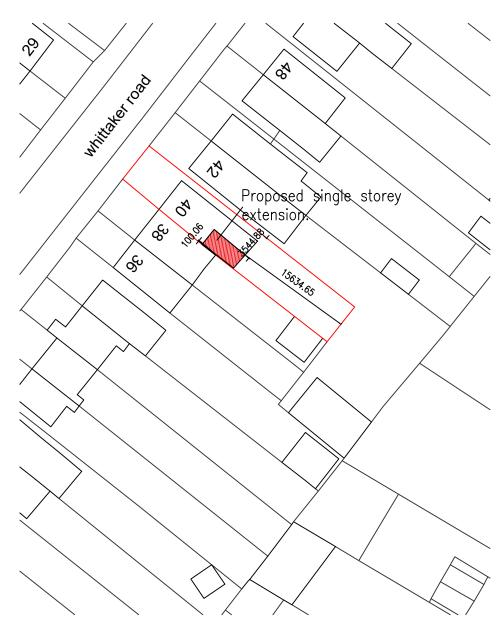
The proposed extension will infill the existing space and not protrude beyond the existing rear building line of number 40, it will be no closer to the existing rear boundary or the boundary with number 42 than the current building. It is placed 100mm away from the boundary fence, and shares the party wall (with neighbour's prior agreement) where abutting the existing extension at number 38
