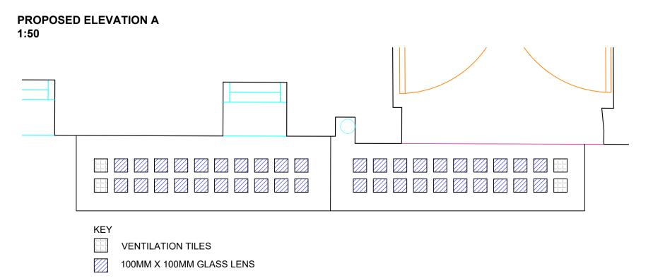
INDICATIVE PAVEMENT LIGHT LENS AND VENTILATOR ARRANGEMENT
