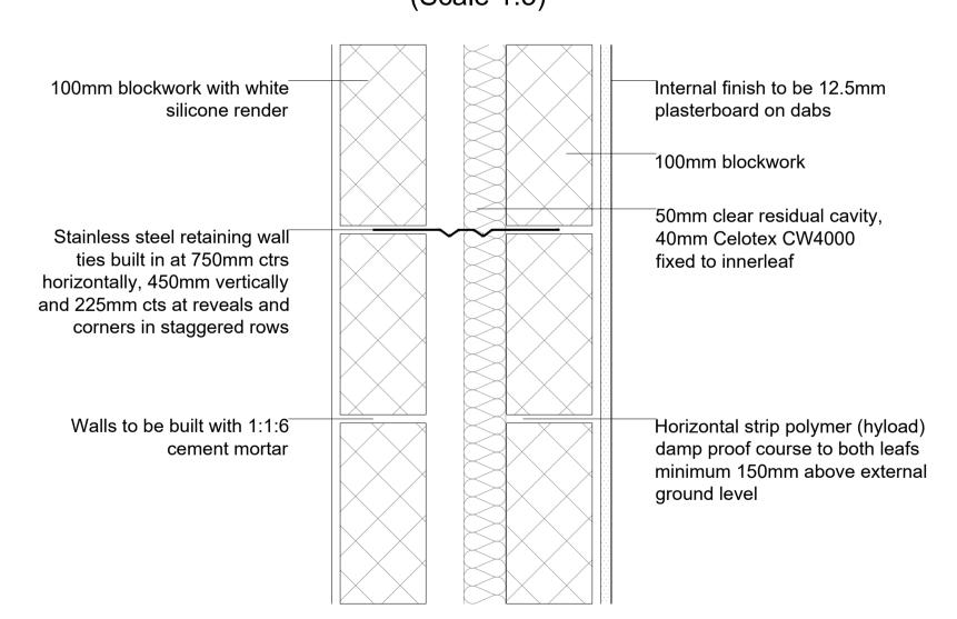
BRICK FILL CAVITY WALL (Scale 1:5)
