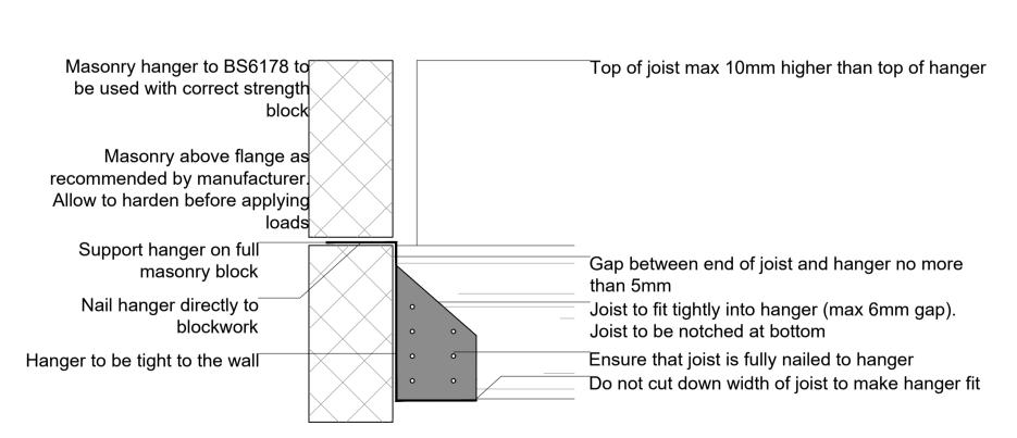
STANDARD MASONRY HANGER (Scale 1:5)
