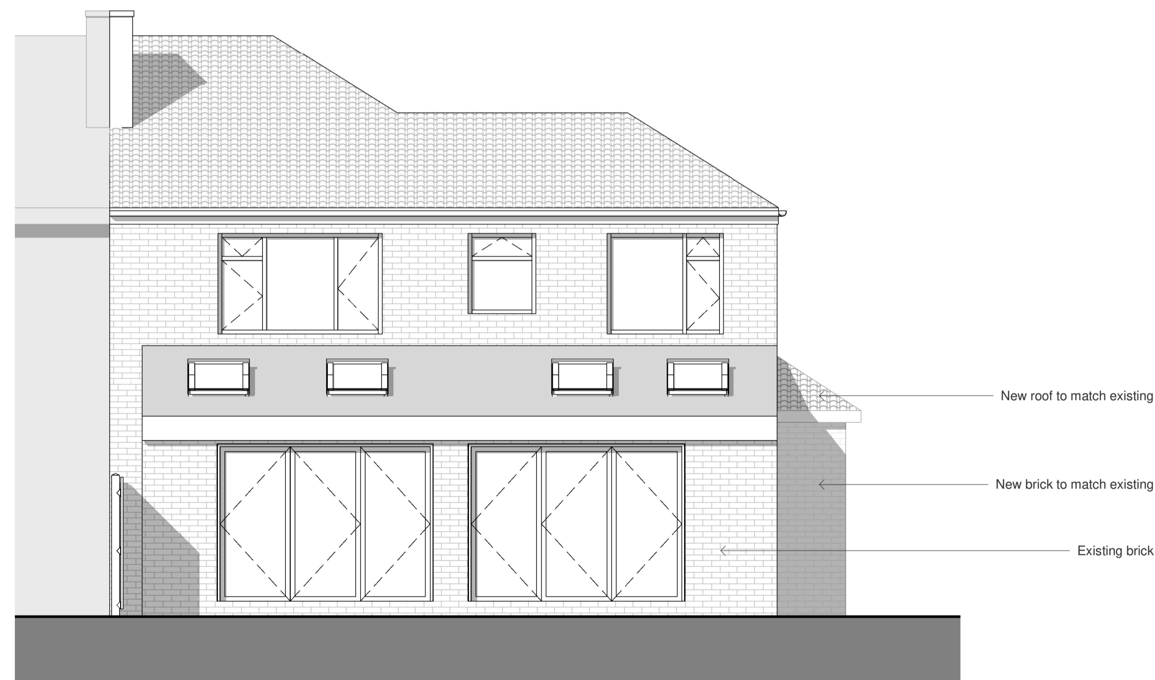
Proposed Elevations - North-West
