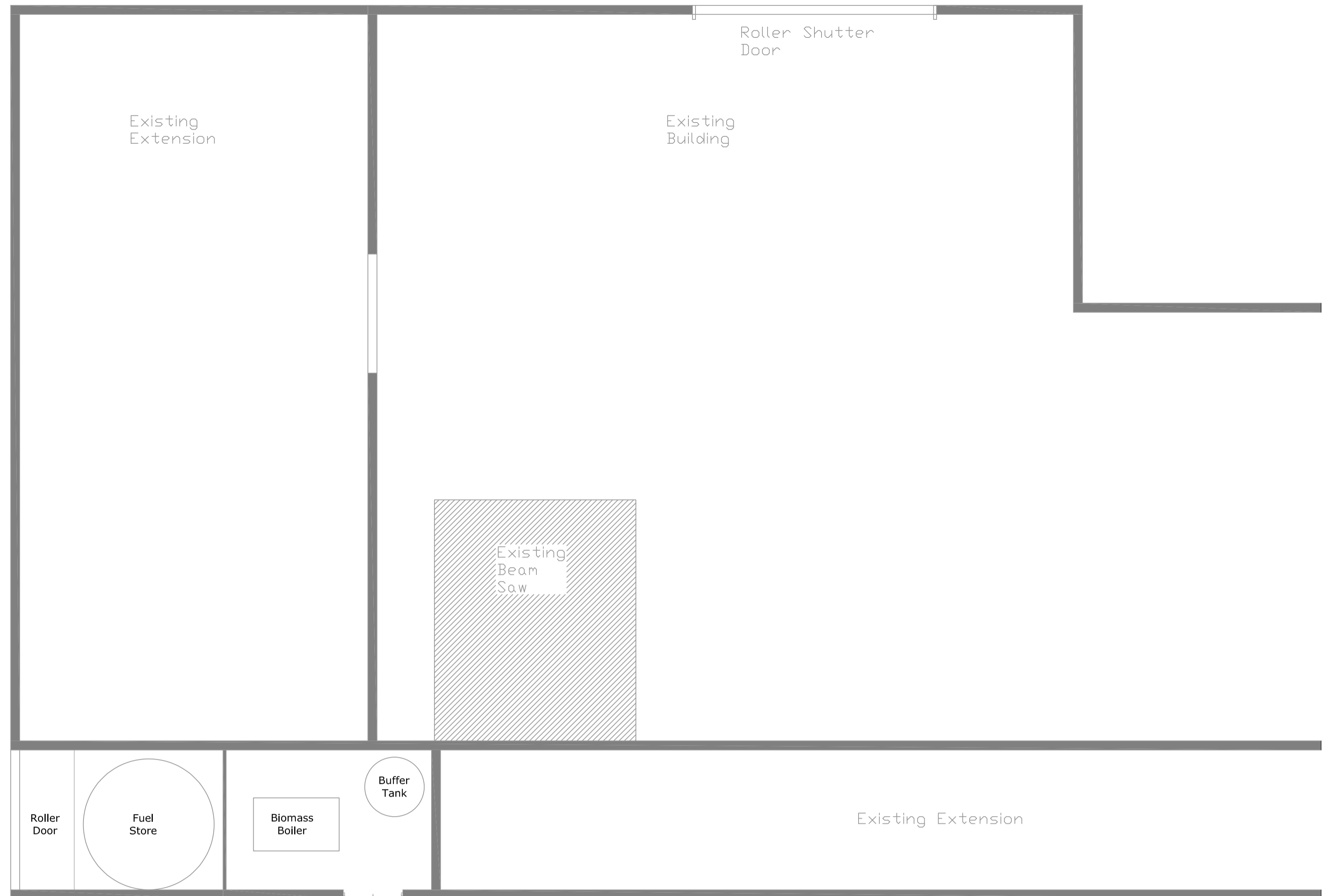
Plan of Building Showing Location of Existing Plant Room and Wood Chip Fuel Store within Existing Building
