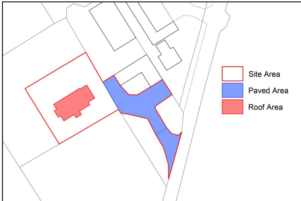
Figure 13. Proposed roof and existing paved areas.
