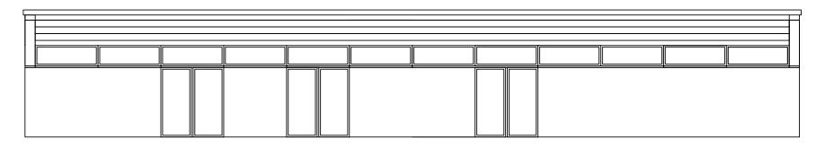
Additional 150mm roof height, New cladding to replace panelling
