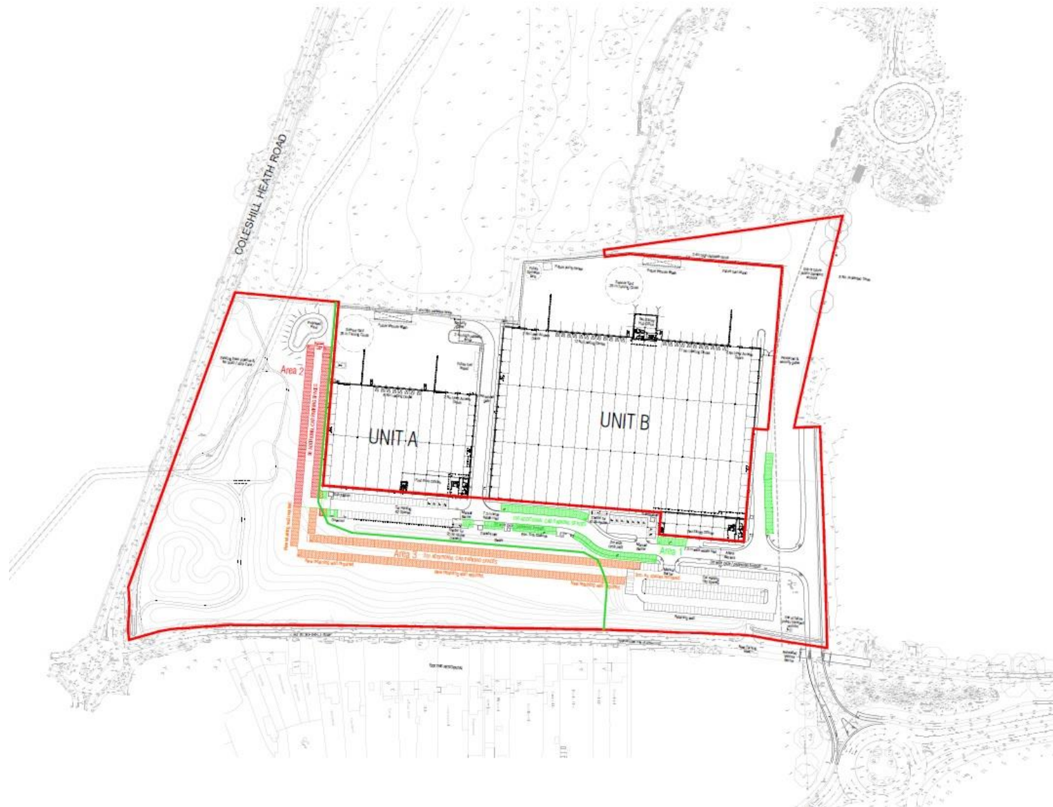
Fig 14. BICKENHILL LINK - Proposed car parking layout- red area 90 spaces, orange area 201 spaces and green area 100 spaces.
