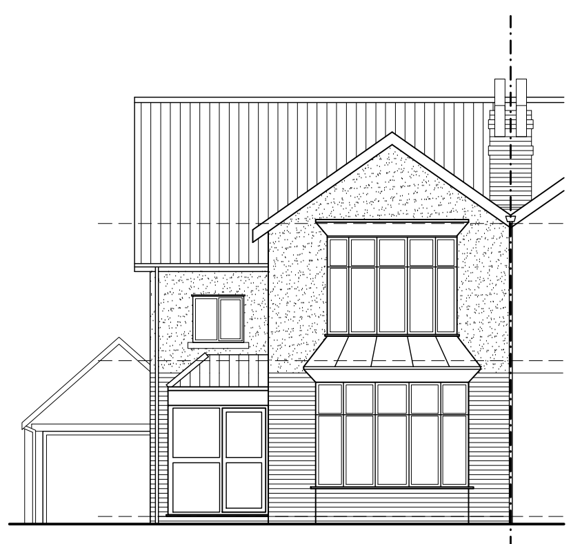
Proposed South Elevation - 1:100
