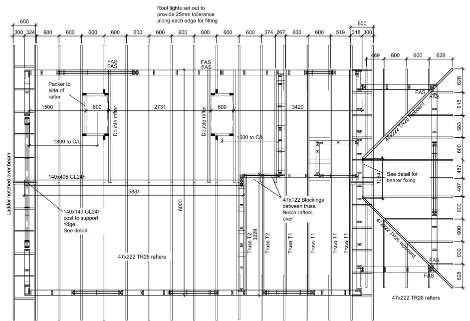
9mm OSB Sarking required to U/side of ALL loose rafters after installation is complete
