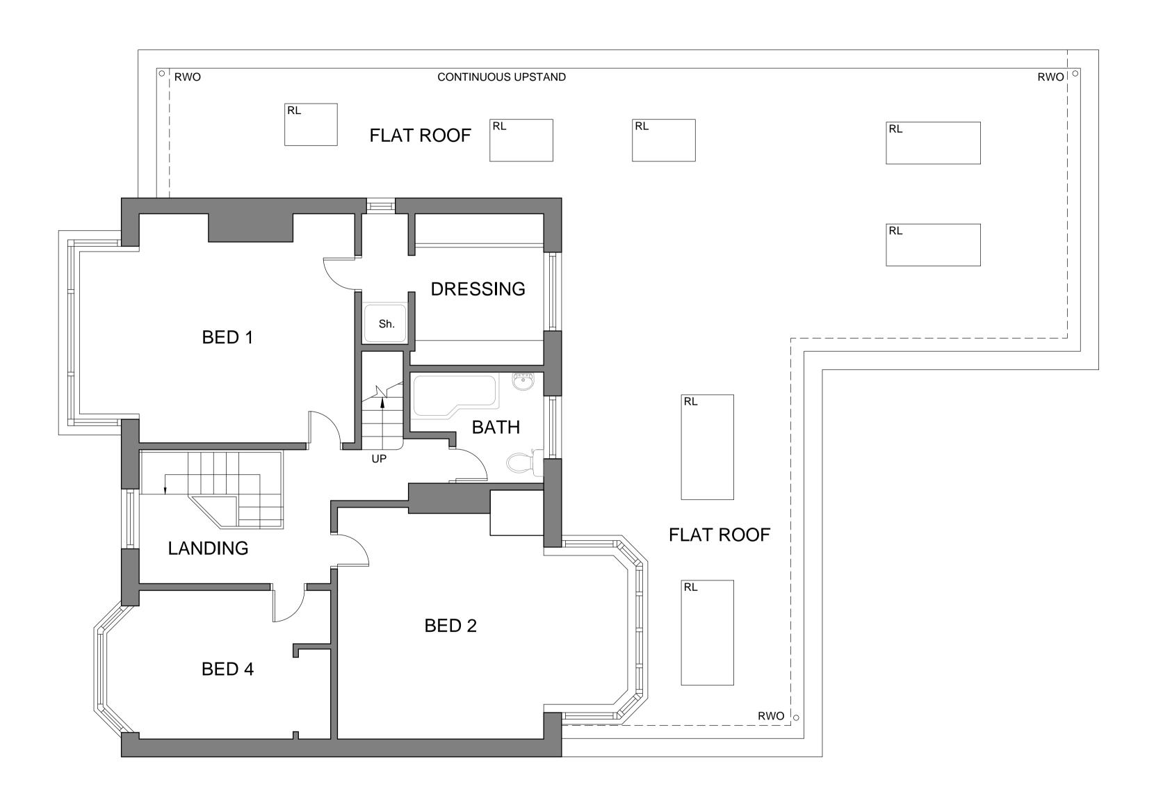
PROPOSED FIRST FLOOR PLAN & GROUND FLOOR ROOF PLAN
