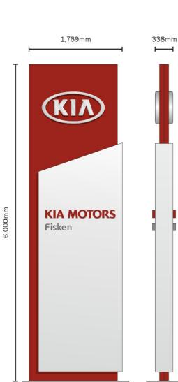
Sign 'D' Scale 1:50 Description: Dealer name sign Materials: aluminium, foamex Illumination: Non-illuminated Sizes: 5,000mm x 960mm Can height for 'F' of 'Fisken' = 360mm Ground level to underside of sign: 4670mm
