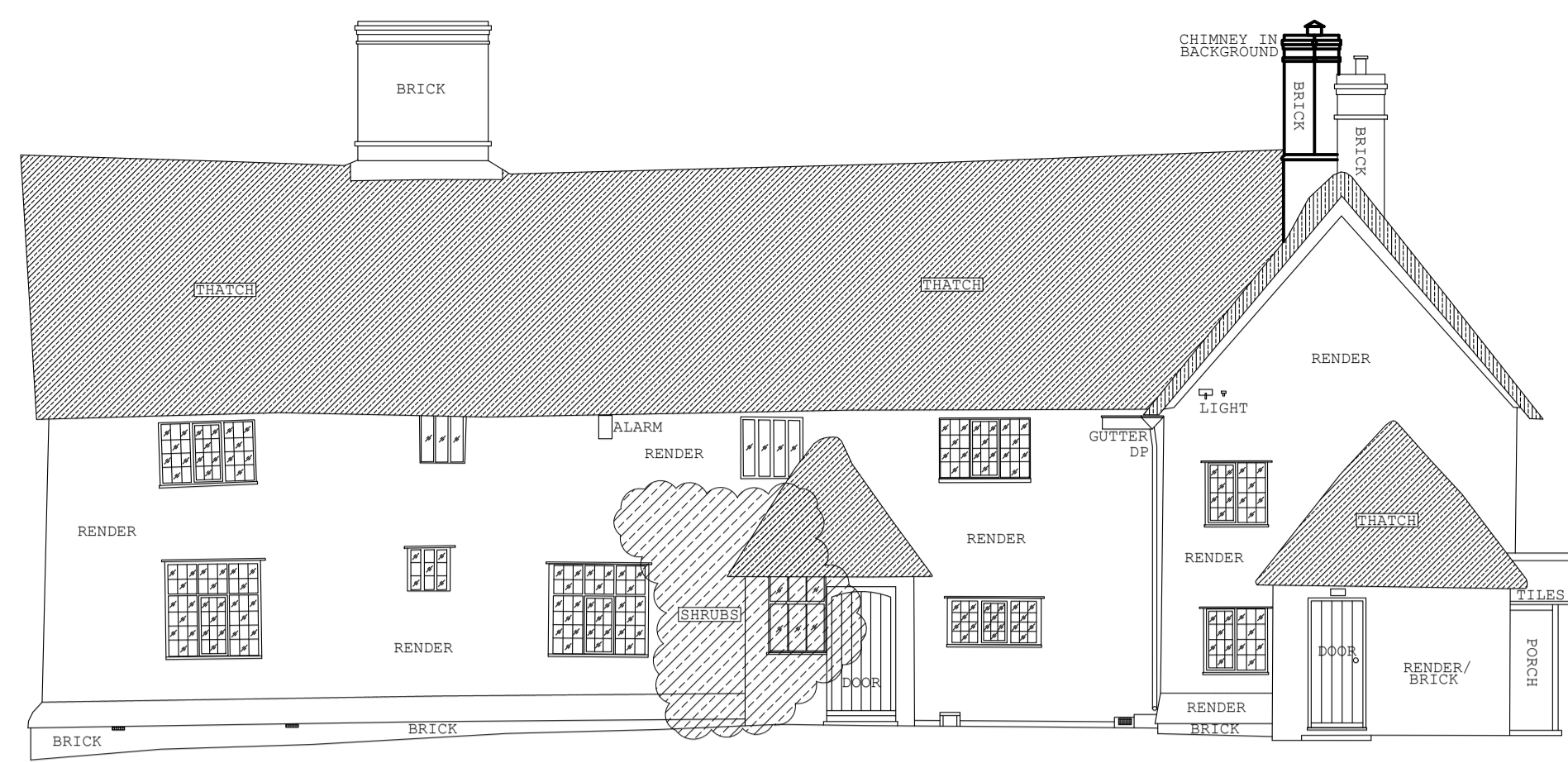
EXISTING SOUTH WEST ELEVATION @ 1:100 SCALE
