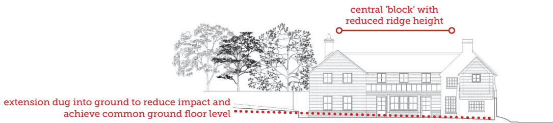
West facing site cross section showing existing Eastern gable end, with new extension to rear
