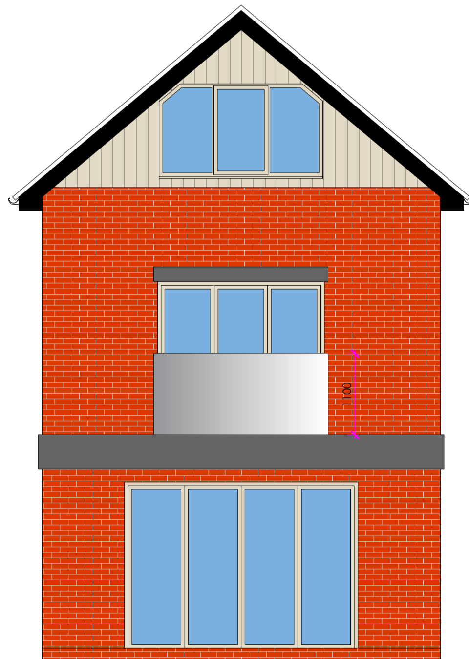
No. 135a - Proposed Rear Elevation
