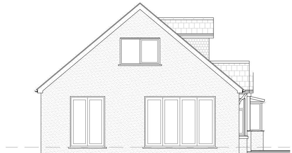
PROPOSED REAR ELEVATION
