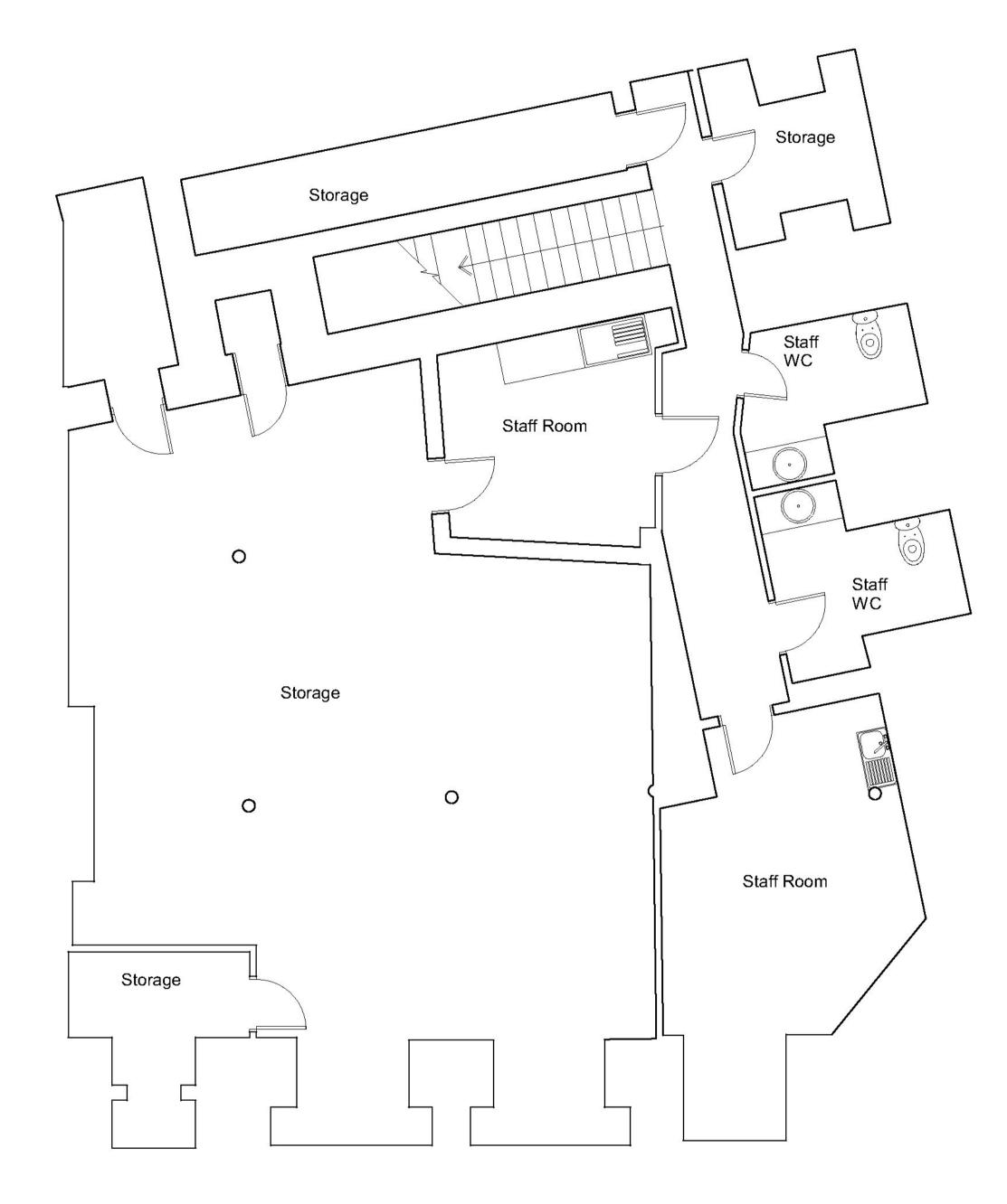
Basement Floor Plan - As Proposed
