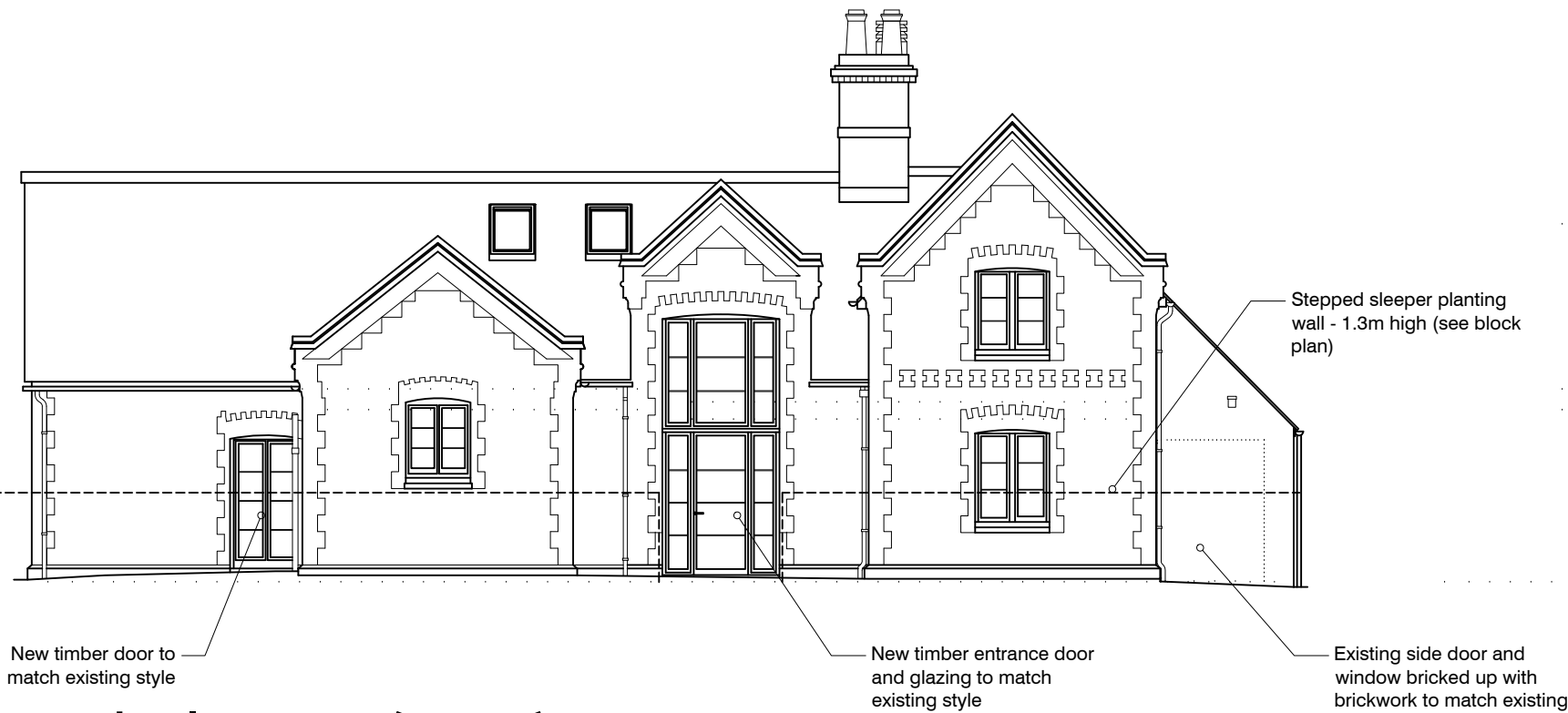
South Elevation (street)
