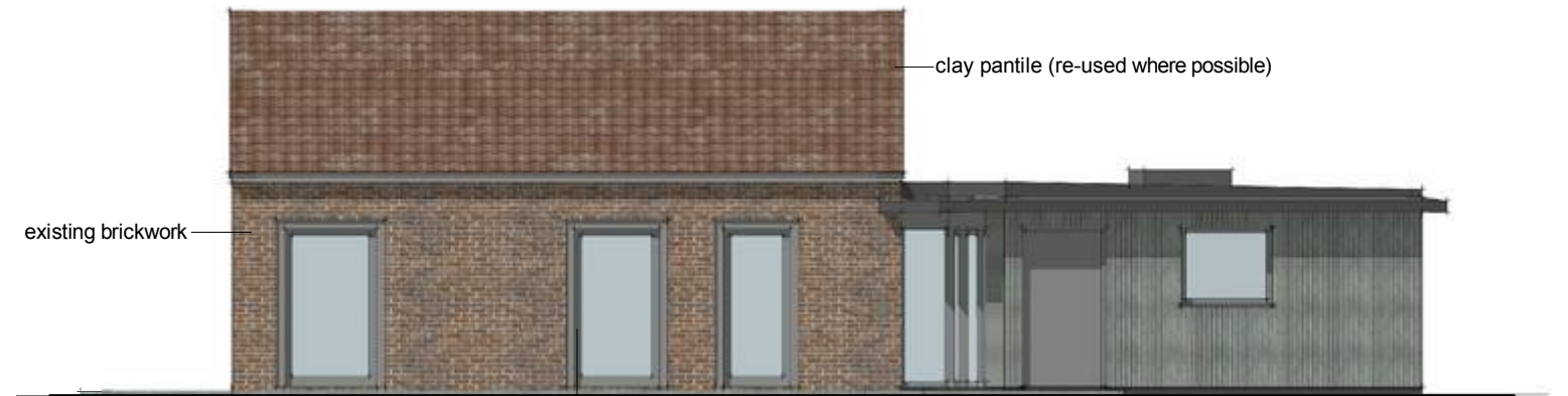
01 Proposed North Elevation scale 1:100 @ A3
