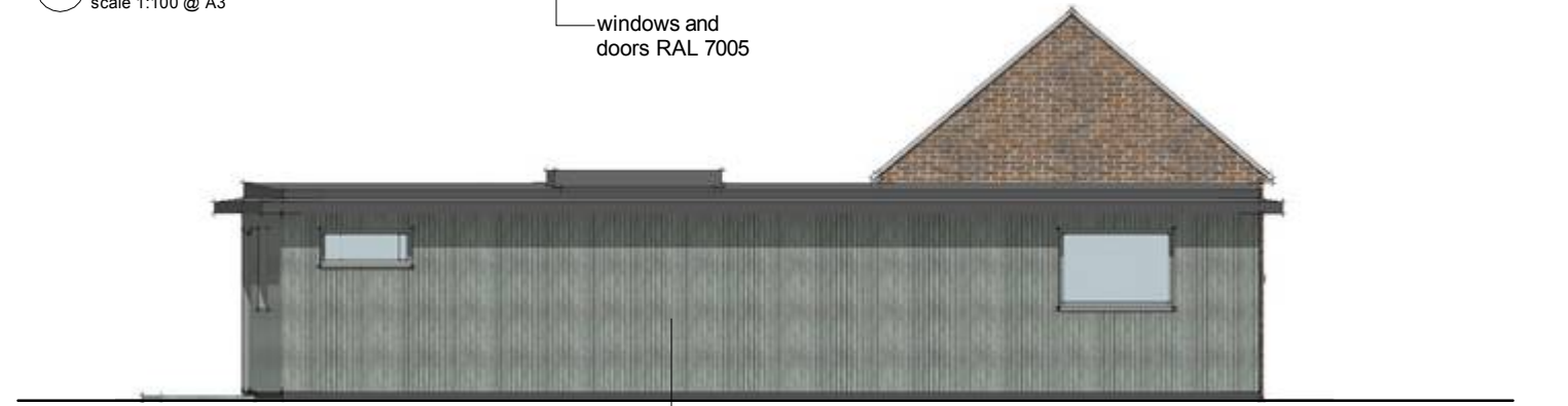
02 Proposed West Elevation scale 1:100 @ A3
