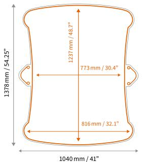
A design which is sturdy, intelligent and attractive. It is compact with a total footprint of only 1040mm x 1378mm; including the rails.
