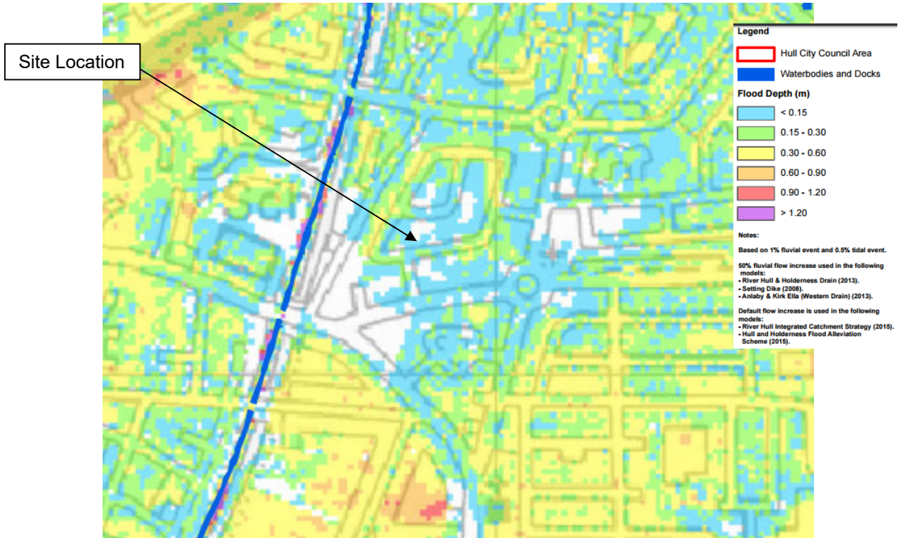
Extract from Hull SFRA – (Fig 3b) Flood depths with defences + climate change & 50% Upper end fluvial flow 5
