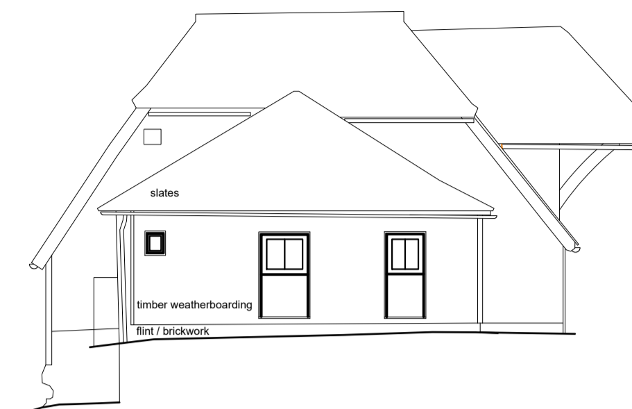
North-West Elevation scale 1:100 @ A1
