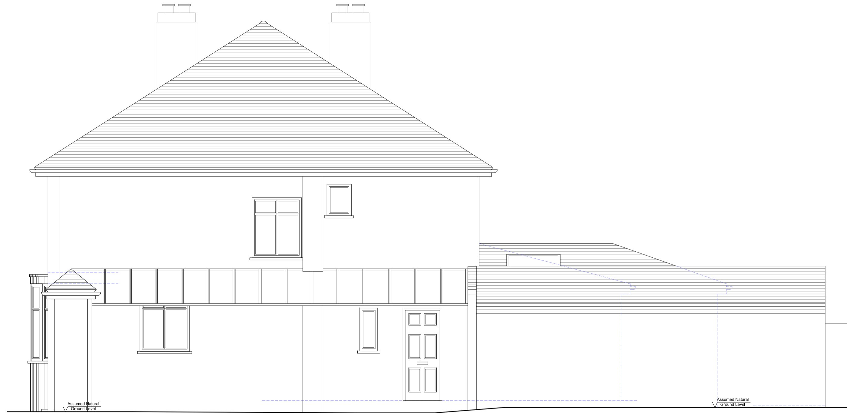
EXISTING SIDE ELEVATION -A-
