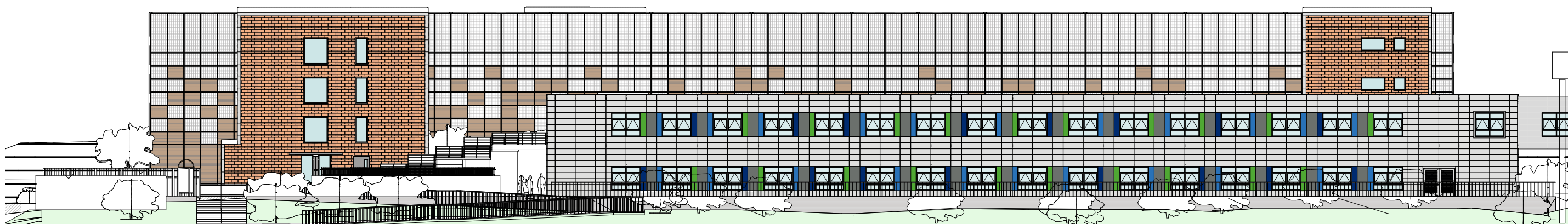
2D elevation study of the south MSCP elevation with the façade of the new ward.
